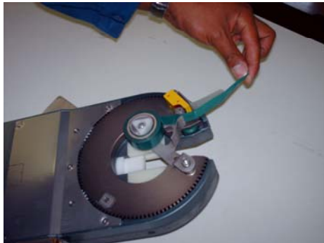
3-Extend the tape with adhesive side opposite at cut blade and set the nut friction tape
