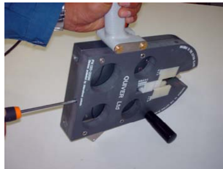
4-Set the three pusher coil size Switch on the main switch on control box
